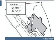
• Fit fuse 15A from the kit in position 3 on the fuse holder.
