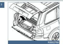
Remove the folding side panel from the left and right-hand side of the cargo compartment.
