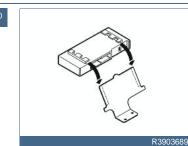
Press the control module in the bracket.
