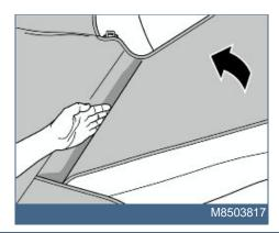
• Fold up the backrests. At the same time insert the dirt cover in the space between the backrest and the cargo compartment floor.
