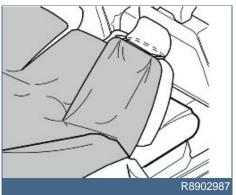
Fold up one of the outer backrests slightly. Thread the strap on the flap over the head restraint.
