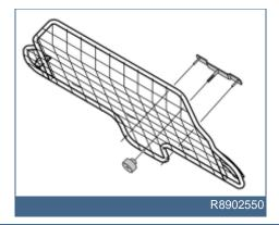
Remove the locking device from the cargo compartment net by unscrewing the knob and pulling it off.
