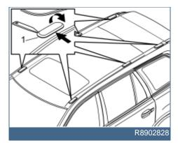
Carefully pry off the six covers (1) using a plastic weatherstrip tool.
