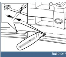
Cut a 2 mm (5/64") wide groove through the plate leading in to the holes on both sides of the cut-out.
