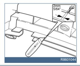
• Cut a 2 mm (5/64") wide groove through the plate leading in to the hole.
