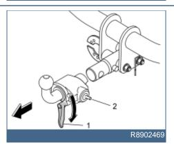
• Remove the tow hitch by turning the handle (1) to the right until a click is heard and the pin (2) is in the outer position. Pull out the hitch.
