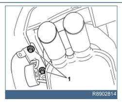
Remove the rear mounting for the silencer and the bracket from the underneath
