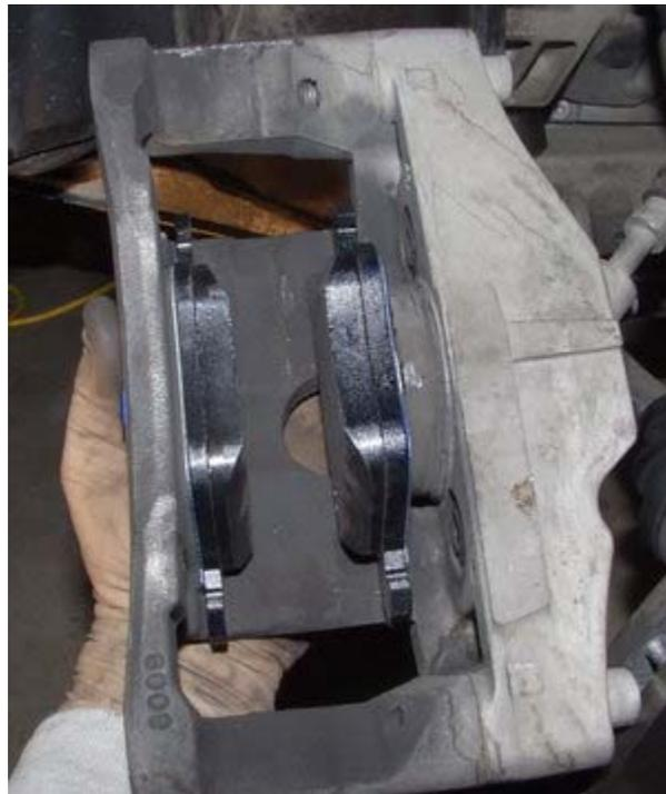
Pad orientation in caliper.
