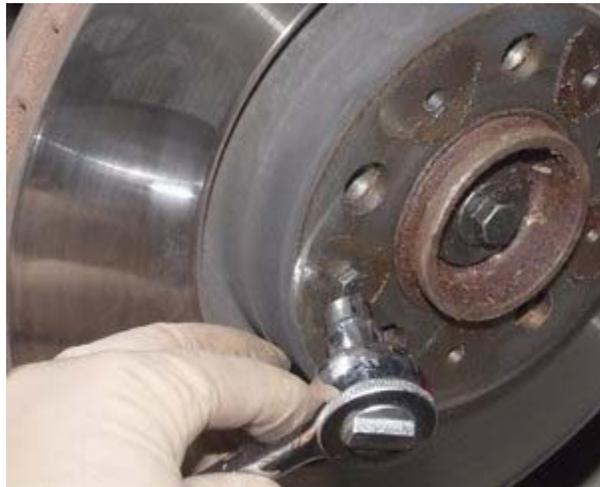
**\*\*Carefully clean the face of the hub to make sure it is free of any debris and the new rotor will sit true.**
