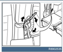
Insert the Velcro strips on the outsides of the cushions through the mounting eyelets positioned in the opening of the cargo compartment. Press the Velcro strips together.
